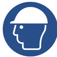
M014 Wear head protection
