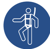
M015 Wear a safety harness
